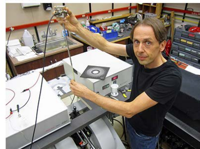
Spin doctor: Christoph Boehme inserts an OLED into a spectrometer
